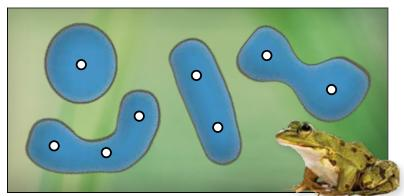
This is a reference to illustrate placement of units to achieve optimal results when aeration is your primary objective. For best results break HP requirements into smaller units and space throughout the water feature.
