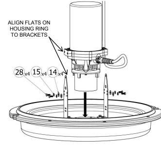
STEP 3 - POSITION UNIT & TIGHTEN BOLTS
